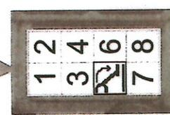
➤ ST"X" FAIL indicates that outrigger n. "X" is not touching the ground.
