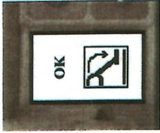
Pressing the green button (number 7) on the remote control the machine start the automatic stabilization procedure. That procedure will be completed only when the display will shows the MACHINE STABILIZED icon (see the picture on the right). Stabilisation is the necessary condition to allow aerial part movements.
